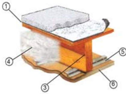
FIGURE 3—SOUND RATED ASSEMBLY INCORPORATING WOOD JOISTS
