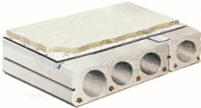
FIGURE 5 — SOUND RATED ASSEMBLY INCORPORATING PRECAST CONCRETE UNITS
