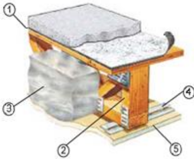
FIGURE 2 — SOUND RATED ASSEMBLY INCORPORATING WOOD TRUSSES
